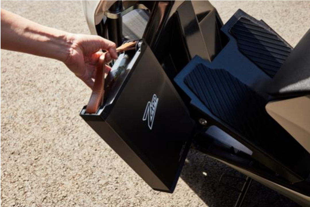
The i300 has a removable battery pack for indoor charging.
