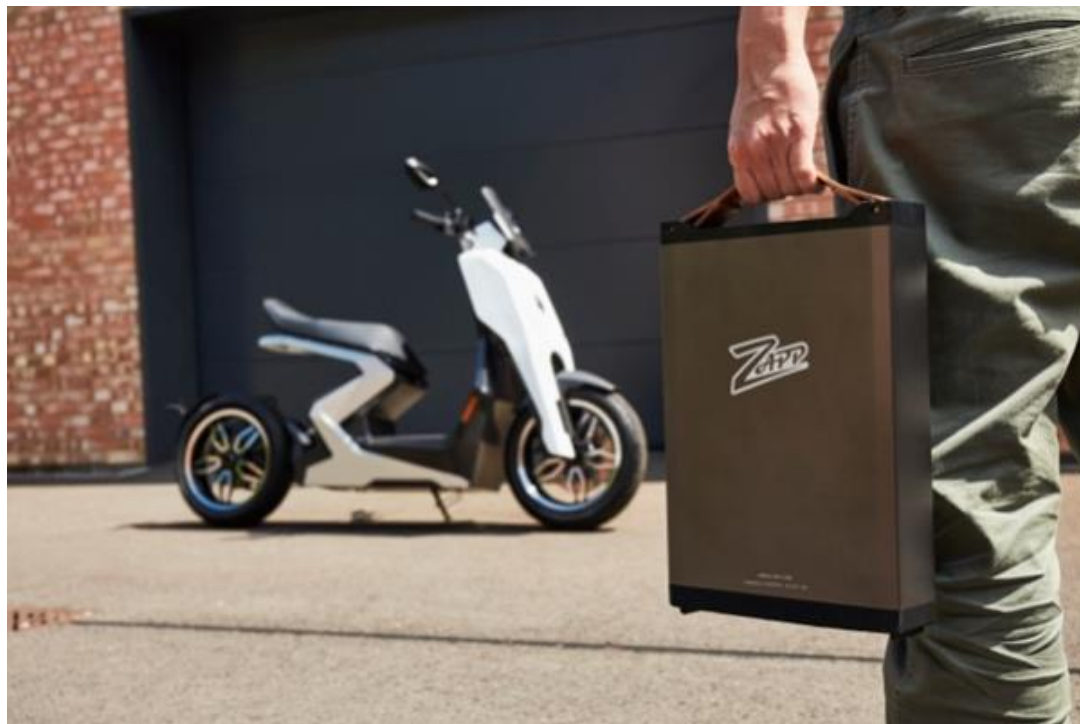
Zapp Electric vehicles i300 scooter view from the side with man's hand carrying removable battery pack
